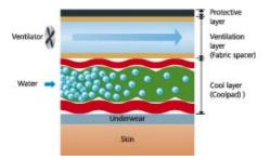
A multilayer system provides active cooling, including ventilation through the fabric spacer.
